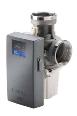
The Brain® can be installed as the final temperature control device before the hot water leaves the plant-room or be used to create control zones within the building to simplify balancing, improve circulation and easily manage a thermal disinfection regime. The Brain® is also a retrofit to existing problematic hot water systems.
