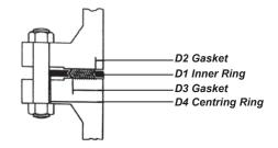
NOTE 1: Inner ring I.D. for 1/2-1" NPS, all ratings not specified by API 601 dimensions shown are manufacturers standard purchaser to specify if different dimension required
