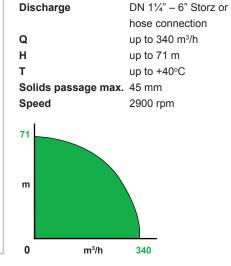
Type: Submersible drainage pump
