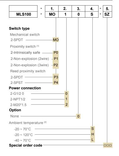
Note 1: By default, two wires intrinsically safe proximity switch(P0) at normally closed status; two wires non-explosion proof proximity switch (P1) at normally open status; three wires non-explosion proof proximity switch (P3) requires customer to select normally open or normally close .
