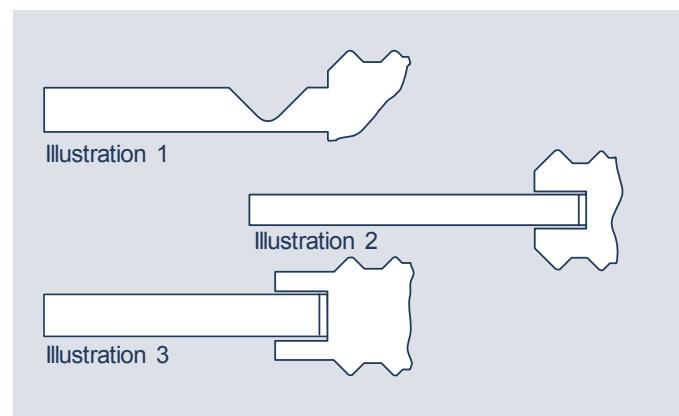
Grooved gaskets are available that conform to works standards WN 100, WN 101, WN 136, WN145 (DIN EN 1514-6), WN 146 and WN 147. Works standards 100 and 101 only contain a sealing width for all nominal pressure levels.
