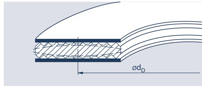
With gaseous media or large differences in temperature between the internal and external diameters, Profile B25A with loose sheet metal central edge should be used.
