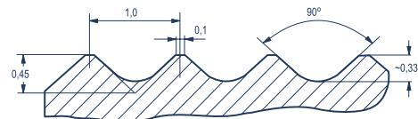
This profiling should be used with gaskets for flange connections with male or female faces or tongue and groove flanges. The minimum requirements are set out in our works standard WN 123.
