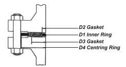
**NOTE 1:** Inner ring I.D. for ½-1" NPS, all ratings not specified by API 601 dimensions shown are manufacturers standard - purchaser to specify if different dimension required.
